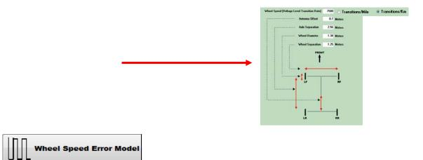
Selection of the Wheel Speed Error Model presents a form in which you may change the default characteristics of the sensor, apply error effects, or setup scheduled "events" which cause anomalies in the output data. If these items are not changed the simulation will generate an exact value data stream. Note the Error model specified here, applies to **both** the <u>Serial Data Output</u> stream as well as the <u>Hardware Pulse Output</u>.
