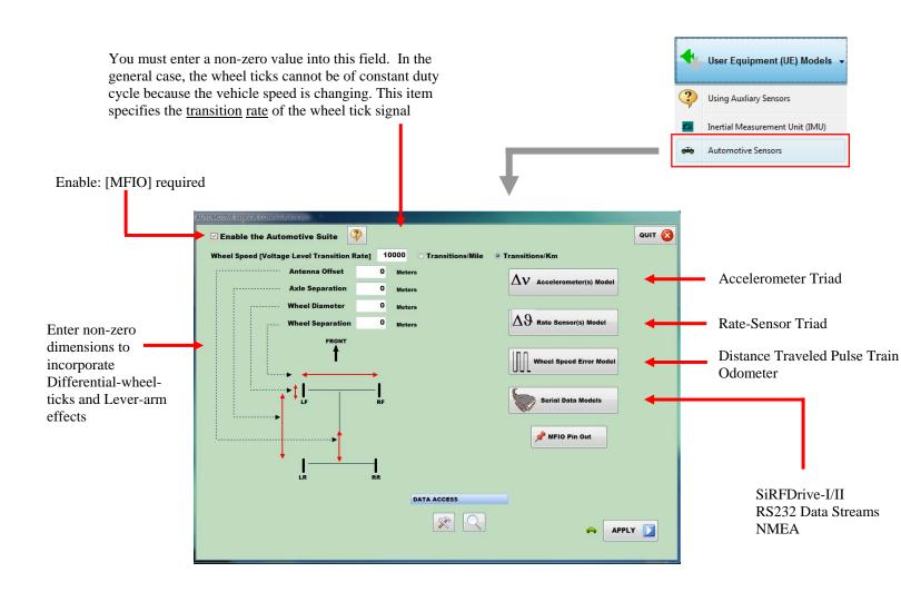
Select the sensor model you wish to configure. If you do not have a Multi-Function I/O [MFIO] expansion card installed in your system, Tapestry will protect the **Enable** control.
