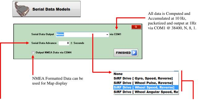
Nominally Serial Data is output "on-time" coincident with the GPS based timing mark.
